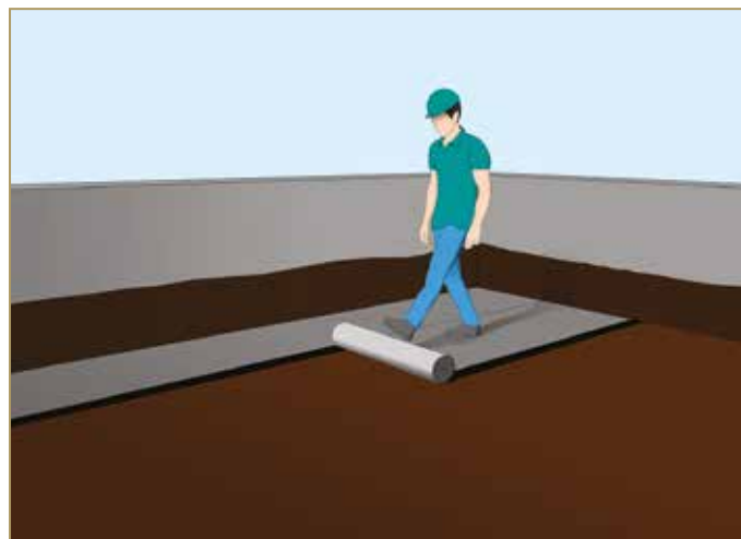
Figura 7.8: Unroll the membrane in its final position
