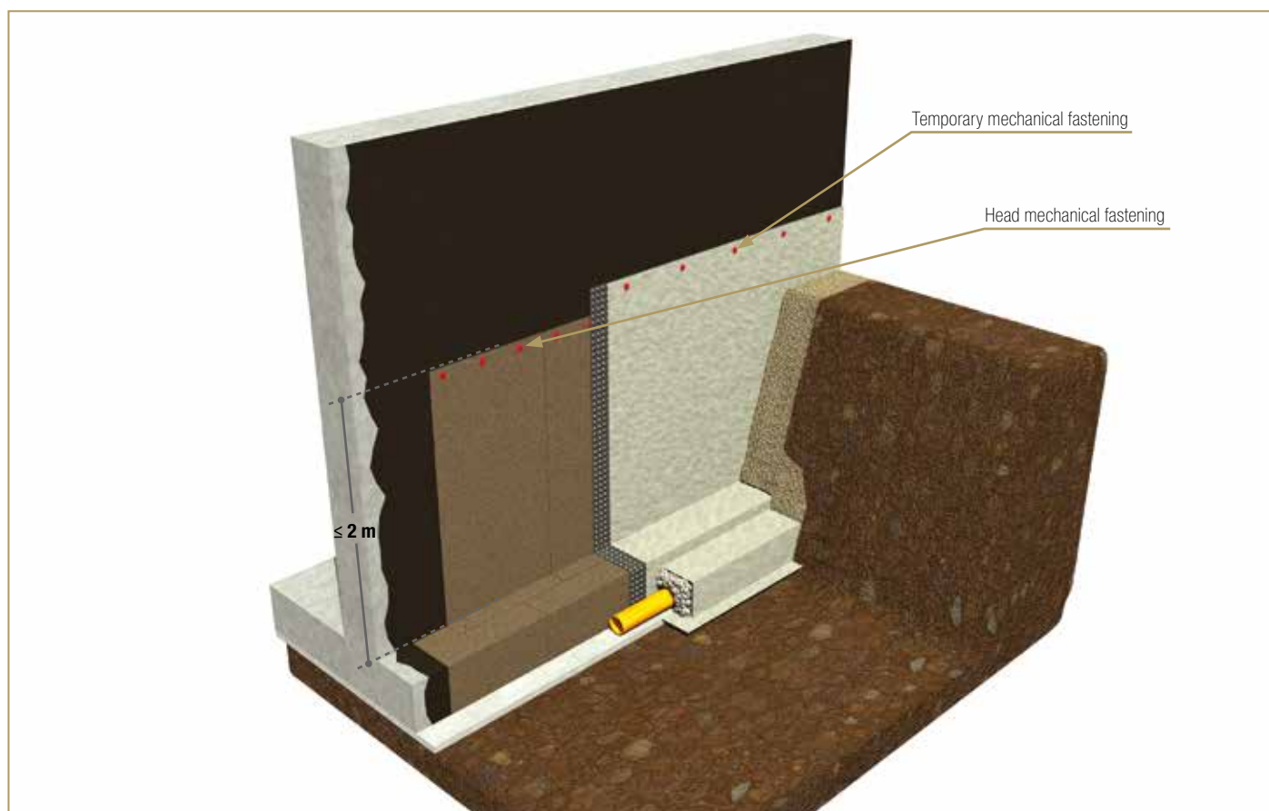
Figure 8.23: First waterproofing phase and associated accessories (first 2 m in height)
