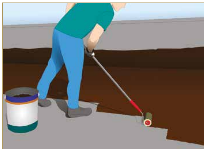
Figure 7.1: Application of the primer
