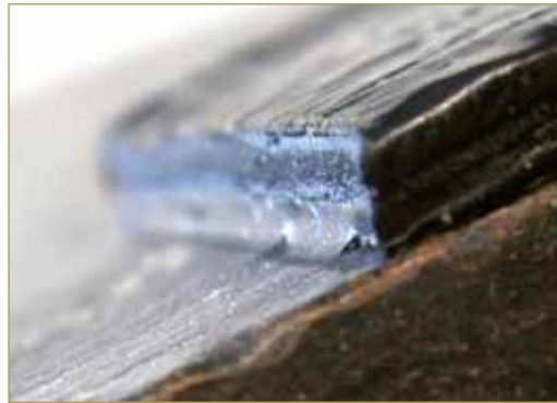
WATER PROOF SHEETS - Determination of high temperature flowing Standard UNI 8202, Part 16
