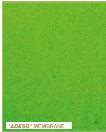
THICKNESS - Fluorescence microscope at 250X magnification. Standard UNI EN 1849-1
