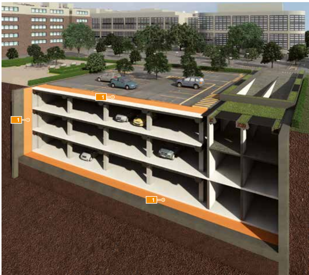
1 Sistema impermeabile Waterproofing system Mapeplan® UG
